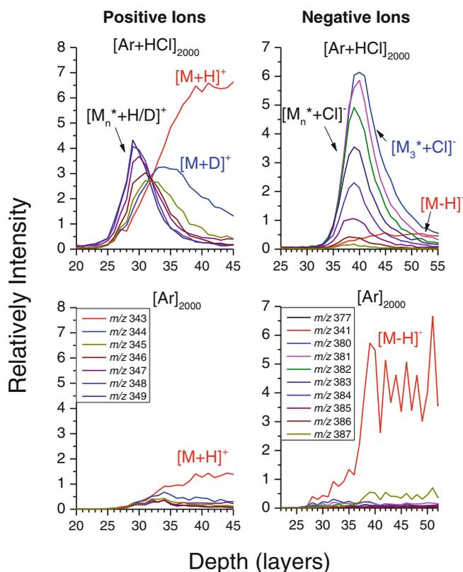
**Figure 4.** Enlarged view of the profiles produced using the HCl doped  $\text{Ar}_{2000}$  GCIB as shown in Figure 3. The notation  $M_n^*$  with  $n = 1-6$  (positive ions) and  $n = 3-10$  (negative ions) describes the exchange of H and D in the trehalose molecule M, where  $n$  hydrogen atoms have been replaced by deuterium
