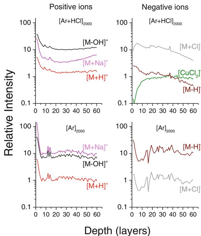
**Figure 2.** Molecular depth profiles of secondary ions emitted from a trehalose film on Cu under bombardment with a HCl doped  $Ar_{2000}$  and a pure  $Ar_{2000}$  GCIB, respectively. The data were taken at 110 K without any addition of water
