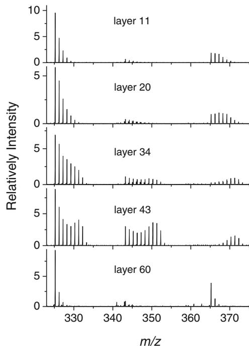
**Figure 6.** Mass spectra measured at the designated points of the dynamical depth profile displayed in Figure 5. The data were taken with the HCl doped  $\text{Ar}_{2000}$  GCIB at 110 K under simultaneous flooding with  $\text{D}_2\text{O}$  at different partial pressures. The three displayed peak groups correspond to the  $[M_n^*-\text{OH}]^+$ ,  $[M_n^* + \text{H/D}]^+$ , and  $[M_n^* + \text{Na}]^+$  (for the definition of  $M_n^*$  see Figure 4) secondary ion signals
